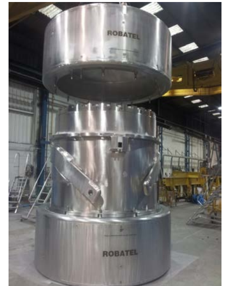
Shipping Cask for Class B and C waste
